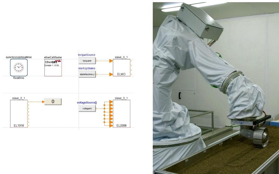
Figure 1. Left: Example model, using code-generated EtherCAT interface blocks to communicate with real-time hardware from within Dymola. Right: DLR Terramechanics Robotics Locomotion Lab (TROLL) with rover wheel attached, controlled via the DLR EtherCAT Library.
